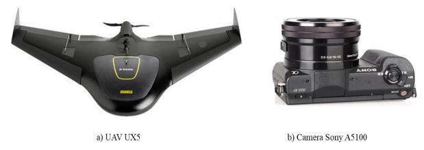
**Figure 3.** UAV and camera attached to UAV.
